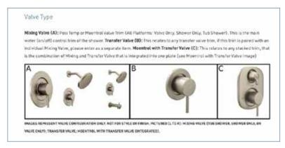
Reference the Valve Type definitions and valve configuration images to help you identify additional applicable products on your wall. Illustrations represent valve configuration only and are NOT for style or finish.
